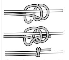
After tying the first end, flip the whole assembly over and repeat the exact same step with the other end
